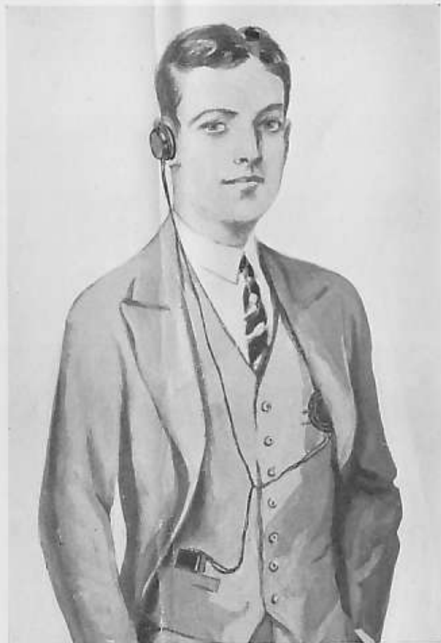
Showing how a man conceals both the transmitter and the battery in his vest pockets.
