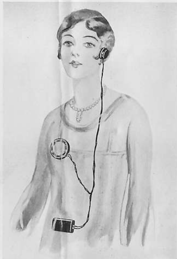
Showing how a woman can completely conceal both the transmitter and the battery beneath her dress.
